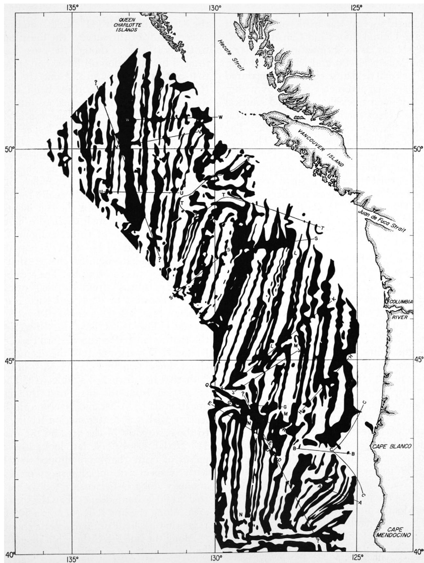
Figure 5.5 Raff and Mason's Figure 1 (1961: 1268). Their caption was simply "Index anomaly map of the total magnetic field. The positive area of the anomalies is shown in black."
